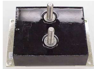
Fig. 5. Photograph of the high-current handling film capacitor.
