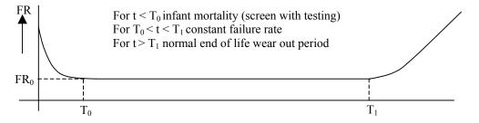
$FR_0$  describes the constant failure rate that can be assumed through the normal service period. The constant failure rate is determined from the accumulation of test hours as required in MIL-STD-690C failure rate "P" at 90% confidence level.
